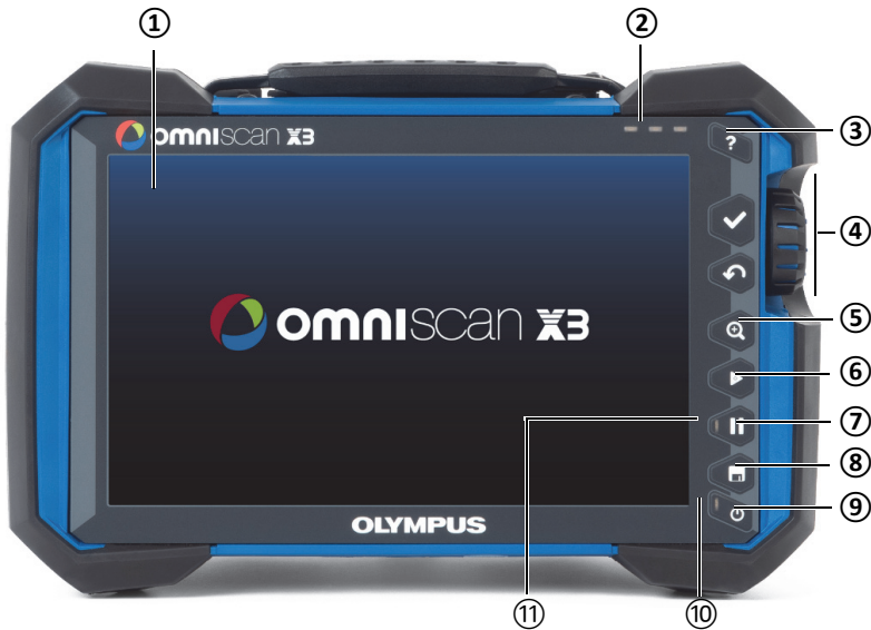
Figura 1-1 Controles del panel frontal del detector de defectos OmniScan X3
