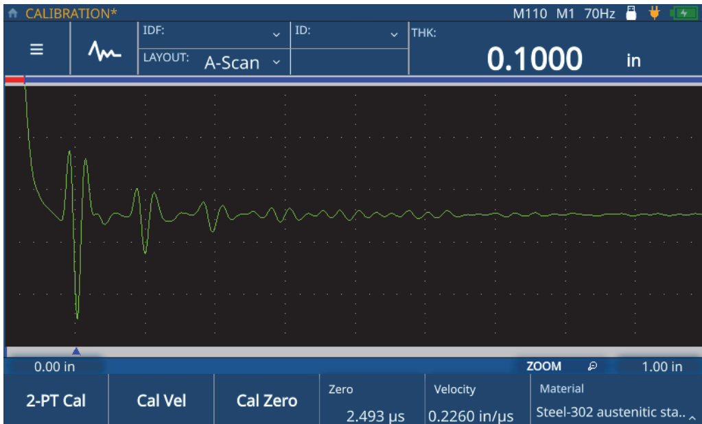
Figure 5-7 Completing Zero Calibration
