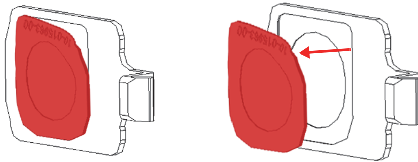
Figure 4-6 Peeling the window (left) and pulling it off (right)
