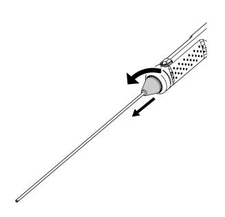
2. Attach the protection sleeve to the rigid scope unit and then fix it by rotating the clamping ring clockwise.
