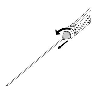
2. Attach the grid extender to the rigid scope unit and then fix it by rotating it clockwise.
