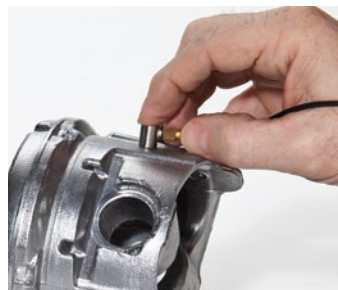
Ultrasonic thickness measurements are accurate, reliable, and repeatable. Instant readings can be achieved from one side of a material, making it unnecessary to cut up or destroy the part.
