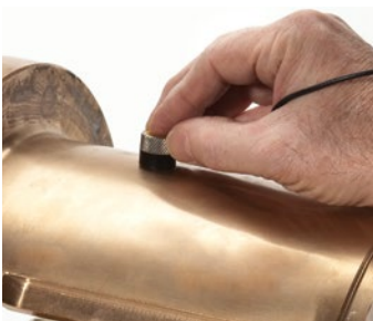
Ultrasonic thickness measurements are accurate, reliable, and repeatable. Instant readings can be achieved from one side of a material, making it unnecessary to cut up or destroy the part.
