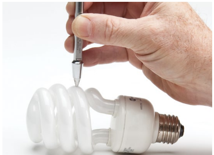
The High Resolution software option enables thickness measurements of up to 0.001 mm (0.0001 in.) resolution.
