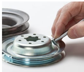
Ultrasonic thickness measurements are accurate, reliable, and repeatable. Instant readings can be achieved from one side of a material, making it unnecessary to cut up or destroy the part.
