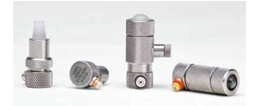
Olympus NDT ultrasonic spotweld transducers are specifically designed to provide optimal performance for nondestructive testing of numerous types of spotwelds, including those used in automotive and industrial applications. Ultrasonic inspection of spotwelds involves the analysis of what is known as the "ringdown" of sound within the weld nugget. Unlike many other direct measurement techniques, spotweld inspection looks at the characteristics of the multiple echoes returned from sound
