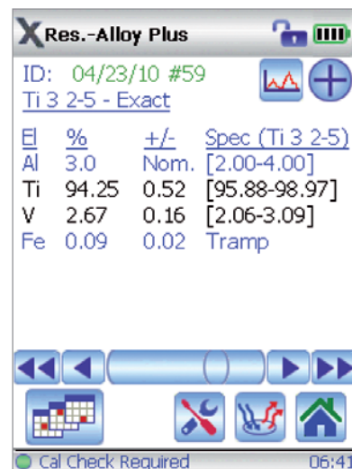
Analysis results display demonstrating nominal value (3% Al) and tramp element (0.09 % Fe) features.
