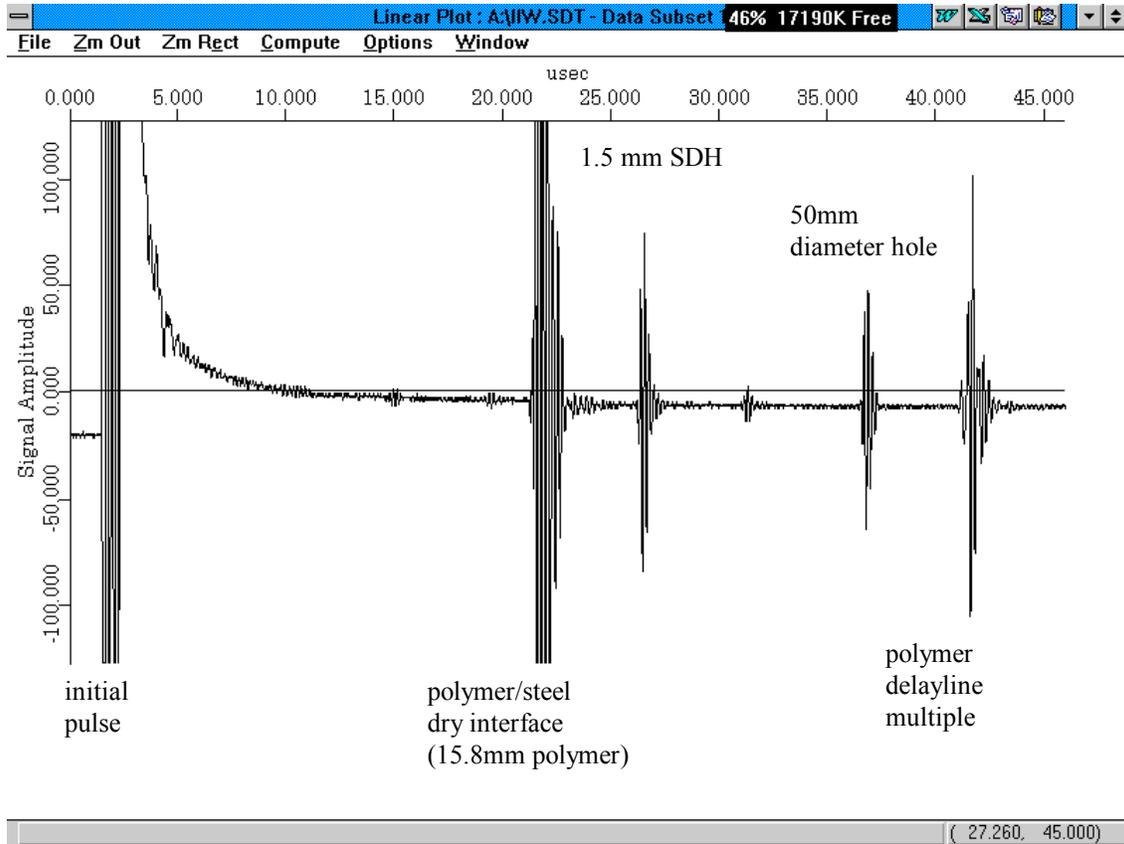
Shown in Figure 2 is the response from the 1.5 mm diameter side drilled hole in an IIW block using a 5 MHz compressional mode transducer. The IIW block to elastomer was a dry interface and a standard gel couplant was used for wetting the transducer which was placed on the 15.8 mm thick elastomer coupling material. A load of approximately 2 kg was applied to the transducer.
