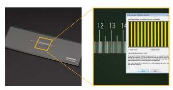
Auto calibration helps eliminate human variability in the calibration process, leading to more reliable measurements
