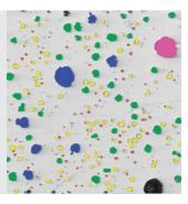
Cast iron solution (Ductile cast iron showing nodular graphite)
