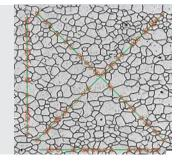
Grain sizing intercept solution (Microstructure with ferritic grains)
