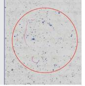
Particle distribution (Particles extracted on membrane filter)
