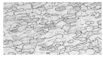
Etched steel microstructure (original image)
