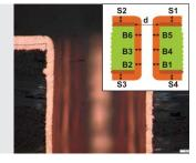
Throwing power solution (Cross section of a through-hole of a PCB)
