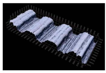
3D surface view (roughness test sample)
