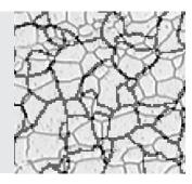
Chart comparison solution (Microstructure with ferritic grains)
