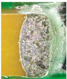
Instant EFI image of a capacitor on a printed circuit board
