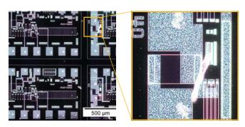
Sharp and high-contrast MIA image of an integrated circuit (IC) pattern (darkfield observation with a 20X objective lens)
