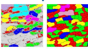
Grain boundary detection with conventional software
