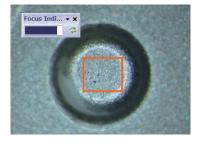
While checking the status of the indicator, adjust the focal point by turning the coarse/fine adjustment knob.
