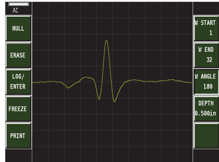
Figure 3-18 Impedance display (left) and external sweep display (right) of flaw at a depth of 0.500 in. in the reference standard
