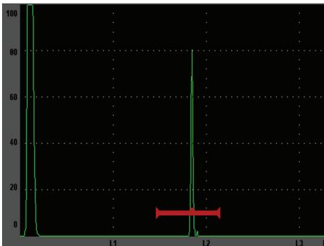
**Leg grid:** displaying vertical lines representing angle beam inspection legs. This mode displays up to 4 divisions, labeled **L1** to **L4**, which represent each half-skip distance of a test piece during an angle beam inspection. The spacing and number of divisions displayed depends on the **Basic > Range**, **Basic > Delay**, and **Trig > Thick** (material thickness) parameters.
