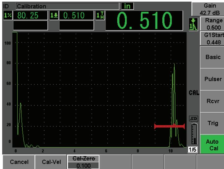
Figure 10-8 Example of a gated signal for velocity calibration
