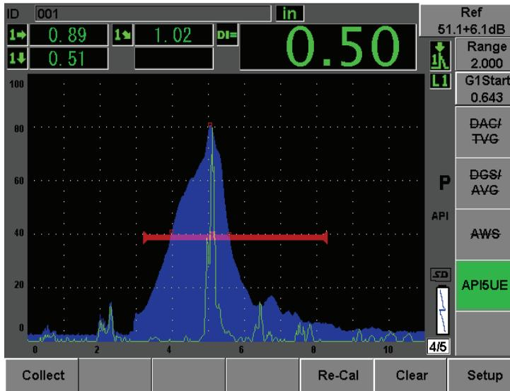
Figure 12-21 Completed API 5UE sizing
