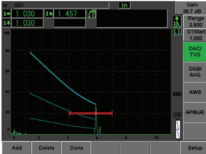
Figure 12-4 DAC Setup one point
