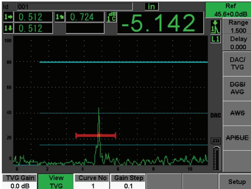
Figure 12-7 Completed DAC curves in DAC view mode
