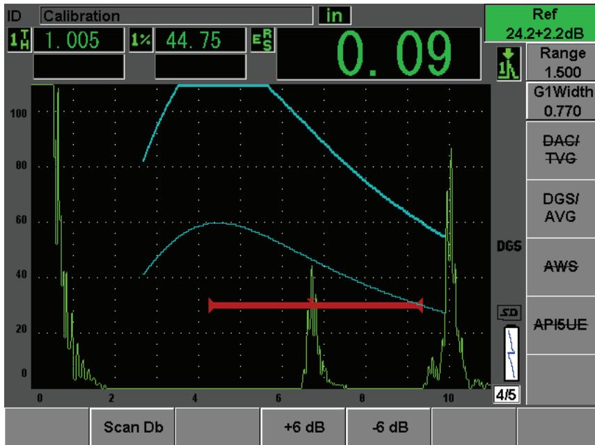
Figure 12-17 Gain curve adjusted DGS
