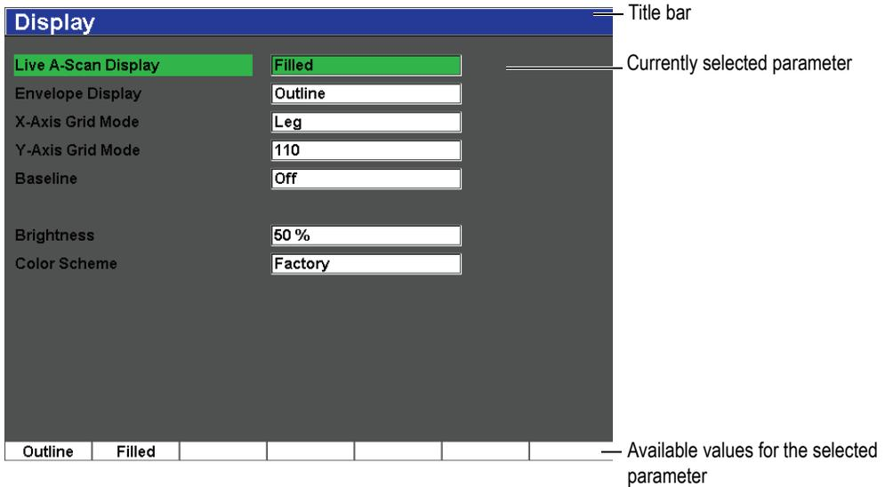
**Figure 5-13 The Display setup page and its elements**
