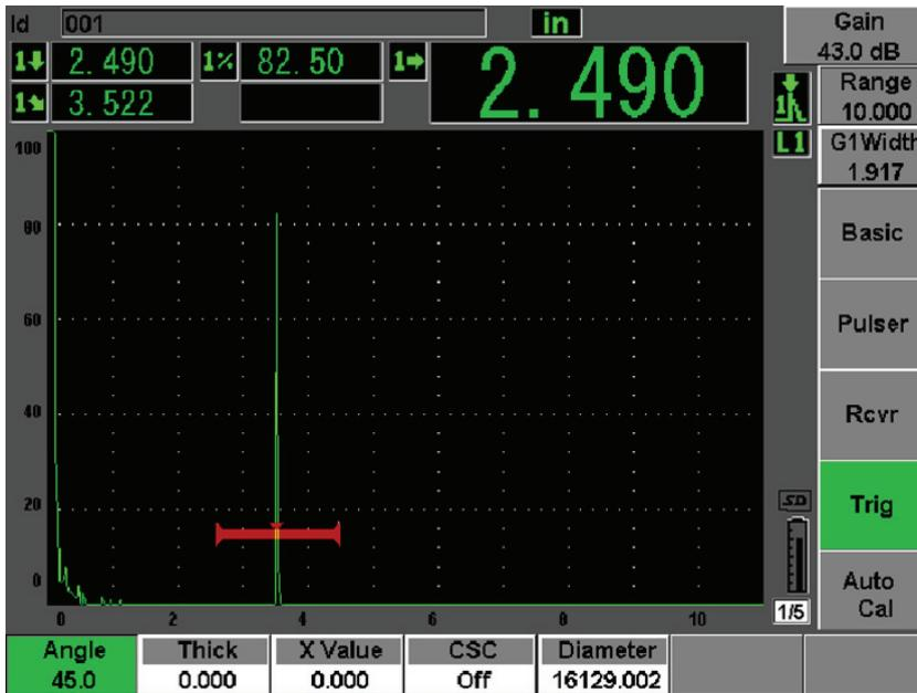
Figure 10-19 Verifying the refracted angle
