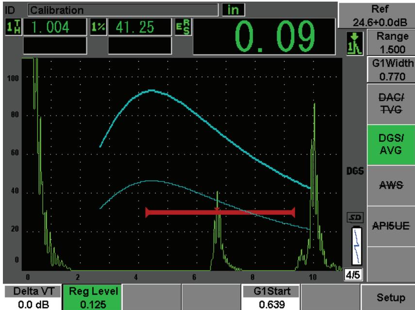
Figure 12-16 DGS/AVG curves on the screen
