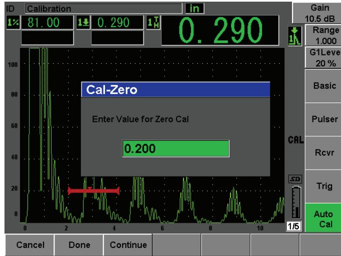
Figure 10-2 Entering the Zero Cal thickness value
