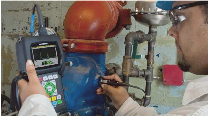
**Figure 1-1** Measuring thicknesses with the 38DL PLUS
