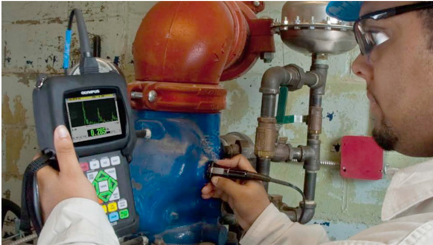
Figure 1-1 Measuring thicknesses with the 38DL PLUS
