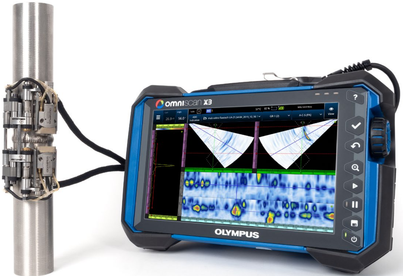
The COBRA scanner on a 0.84 in. OD pipe with two A15 PA probes with an OmniScan X3 flaw detector displaying two PA groups with sectorial scans and C-scans.
