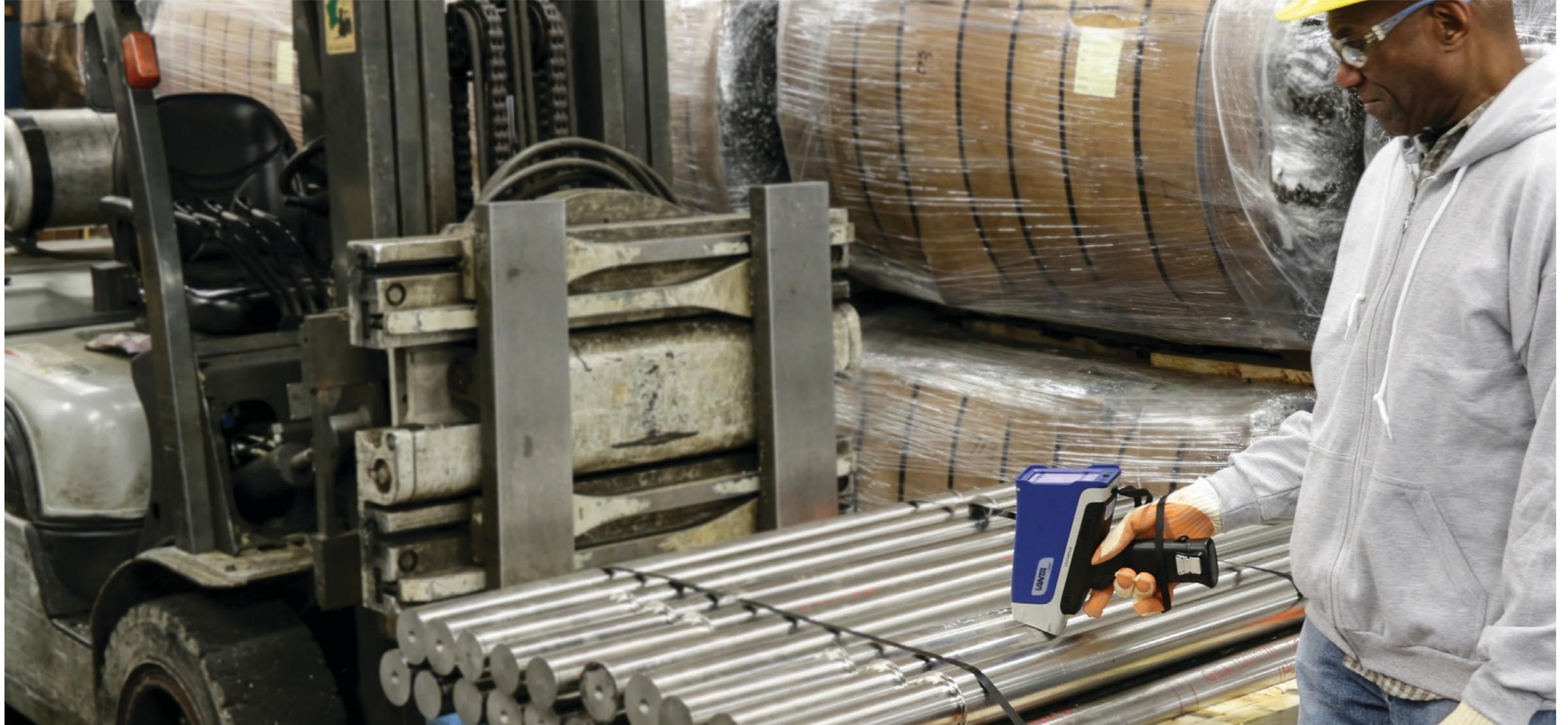
As the price of recycled metals fluctuates, identifying alloy grades quickly and easily is essential for profitability. Vanta™ handheld XRF analyzers for scrap sorting provide reliable identification in seconds for most alloys and pure metals.
