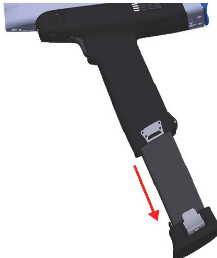
3. Align the contacts of a fully charged battery with the contacts in the Vanta handle, and then insert the battery into the handle.
