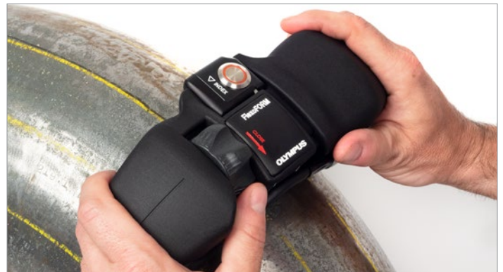
FlexoFORM scanner performing C-scan mapping on an elbow using an integrated encoder and indexing button.
