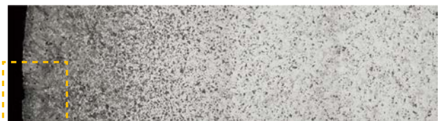
Depth and condition of carburizing can be identified.
