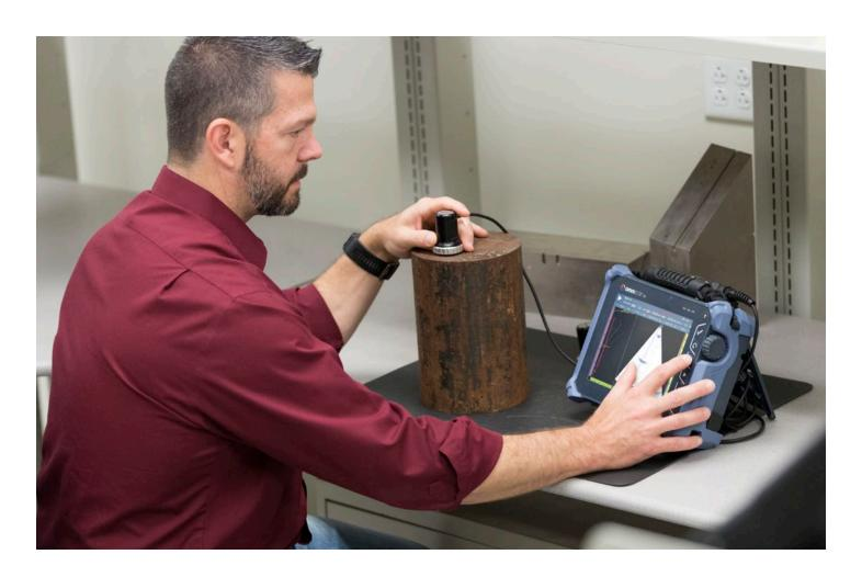
MXU software version 4.4 incorporates the distance gain sizing (DGS) method to streamline your inspections when using an OmniScan® MX2 or SX flaw detector.
