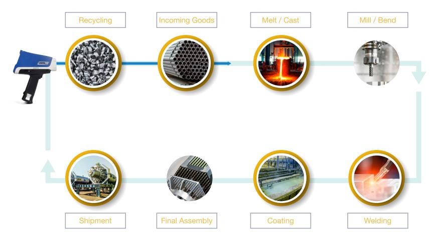
\*Vanta analyzers are used in 6 of the 8 process steps
