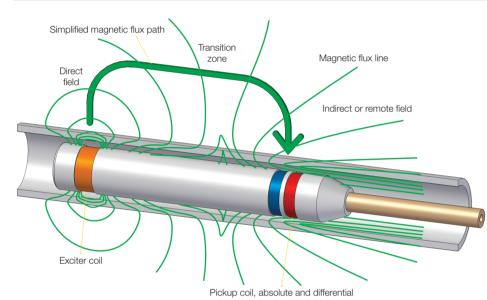
Remote field testing is a through-wall transmission technique, and the probes are used to inspect ferromagnetic tubing, such as carbon
