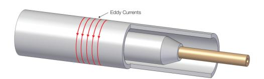
The magnetic field penetrates the tube wall and generates opposing alternating currents in the material. These currents are called "eddy currents."
