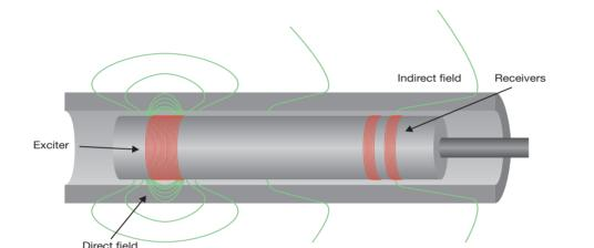
The indirect field is diffused outward through the tube wall; it then propagates along the tube axis and is then rediffused back through the tube wall.
