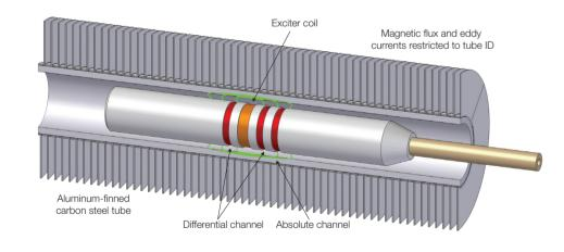
Near field testing for fin-fan tubing relies on a simple driver-pickup eddy current probe without requiring an external reference coil. It is designed to provide very simple signals for analysis. The probe measures the lift-off or fill factor and then converts it into amplitudebased signals.
