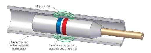
Two coils are excited with an alternating current, producing a magnetic field around them.
