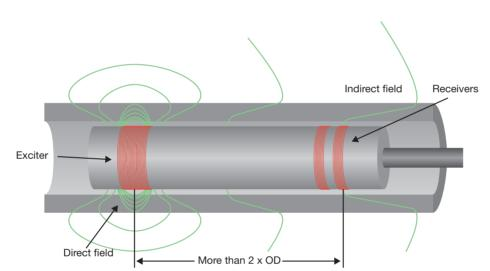
The zone in which the indirect field is dominant is called the remote field zone. This zone is present at a distance greater than two tube diameters.
