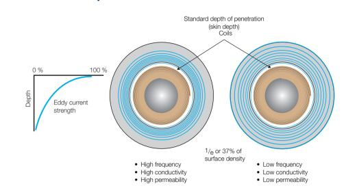
The density of eddy currents in a material is not constant. The density is greatest near the coil and declines as it penetrates the material.
