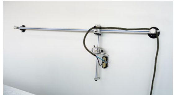
GLIDER semi-automated 2 axis scanner inspecting a wind blade
