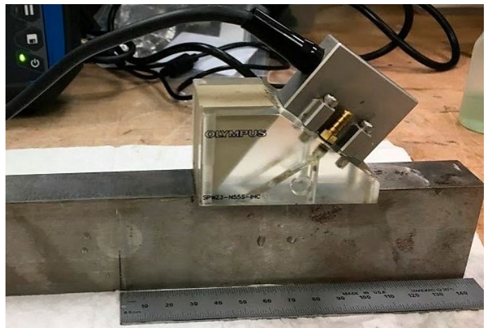
Figure 2—Olympus linear array probe installed on a Rexolite wedge on the SENB specimen
