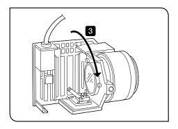
3 Tilt the lamp socket in the arrow direction by 90°.
