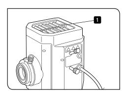
Attaching the mercury burner
