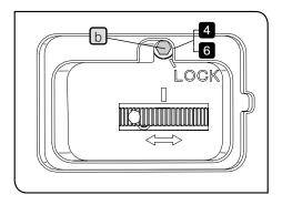
4 Loosen the screw b to unlock.
