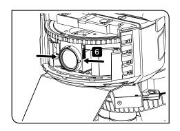
6 Hold the both sides of the inserted fluorescence mirror unit between the thumb and the pointing finger, and swing it from side to side lightly to confirm that the fluorescence mirror unit is secured firmly. Without this operation, the fluorescence mirror unit may be attached being tilted.
