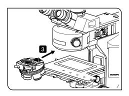
Insert the nosepiece from the front side along the nosepiece mounting dovetail of the reflected light illuminator, and push it until it touches the end. When attaching the coded nosepiece, put the cable a for the nosepiece through the cable hole b on the top of the microscope frame, and put it out to the back of the microscope frame.
