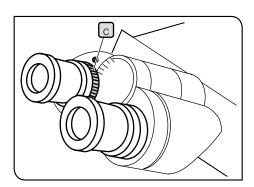
When the observation tube is equipped with the interpupillary distance adjustment ring c
