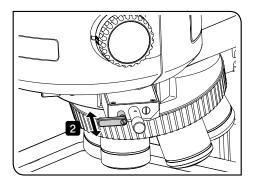
2 When using the DIC slider U-DICR, slide the selection lever depending on the objective to use.
