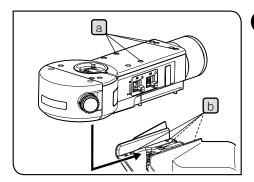
This picture shows the procedure to attach BX3M-RLAS-S. The same procedure applies when attaching other reflected light illuminators.
