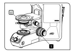
1 Turn the coarse focusing knob to lower the stage holder c sufficiently.
