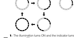
1: The illumination turns ON and the indicator turns ON in blue. 2 Turn the dial c to change the illumination position. The illumination position shifts in the rotated direction by one scale at a time.
