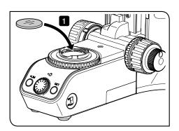
Inserting the filter in the filter mount
