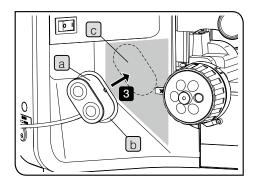
This picture shows the procedure to attach the hand switch for motorized nosepiece (BX3M-HSRE). The same procedure applies when attaching the hand switch for exposure (U-HSEXP).
