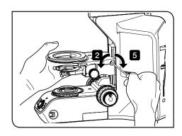
2 While holding the stage holder, loosen the clamping screw of the stage holder.
