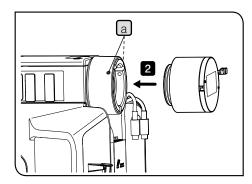
This picture shows the procedure to attach the reflected LED lamp housing (BX3M-LEDR). The same procedure applies when attaching other light sources.
