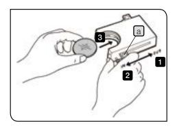
Inserting the filter in the filter cassette
