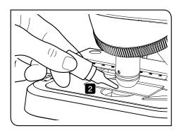
Apply the specified oil (immersion oil) to the tip of the oil immersion objective. Otherwise, the observation image can not be brought into focus.
