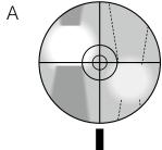
9 Turn the collector lens focusing knob to project the arc image on U-CST. (Picture A)
