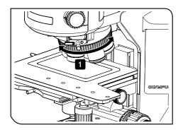
NOTE When selecting the objective, be careful not to collide with the sample.
