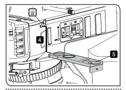
The picture shows the insertion parts of BX3M-URAS-S. The same insertion parts are also provided to BX3M-RLAS-S or BX3M-KMA-S.
