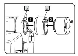
This picture shows the procedure to attach the reflected LED lamp housing (BX3M-LEDR).
