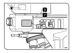
3 Insert a stick with a fine point, such as a precision screwdriver, etc. in the notch a and catch the cover to remove it.
