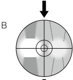
Turn the burner centering knobs to move the arc image to the center of the right (left) half of the field of view. (Picture B)
