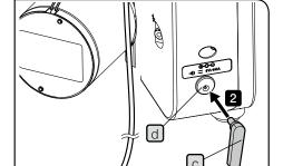
2 Insert the different AC adapter plug c firmly in the AC adapter jack d of the microscope frame.
