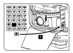
7 Insert the indicator sheet corresponding to the fluorescence mirror unit which was inserted in 5 in the inscription pocket c. The indicator sheet is provided with BX3M-URAS-S.
