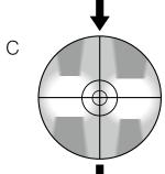
Insert the Allen screwdriver in the mirror focusing screw on the back of the lamp housing and turn it to bring the mirror arc image into focus. (Picture C)
