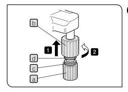
Adjusting the tension of the X-axis knob and the Y-axis knob
