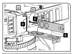
The picture shows the insertion parts of BX3M-URAS-S. The same insertion parts are also provided to BX3M-RLA-S or BX3M-KMA-S.
