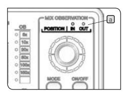
The state whether the MIX slider for reflected light observation is engaged in or removed from the light path can be checked by the POSITION indicator (a) of the hand switch (BX3M-HS).
