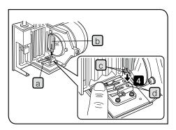
4 While pressing down the bulb fixing lever a, hold the halogen bulb b wrapped with gauze, etc. and insert the terminal c until it touches the pin position d. Place the bulb fixing lever a carefully to the original position to
