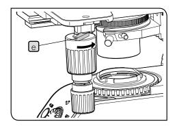
TIP If it is too tight to raise the Y-axis knob b in 1 lock the stage movement with the Y-axis lock lever e once, and turn the Y-axis knob b to raise the Y-axis knob.
