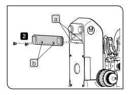
Align the screw holes a (2 positions) on the bottom of the microscope frame with the mounting holes b (2 positions) of the overturing prevention plate, and tighten the provided screws to secure the overturing prevention plate.
