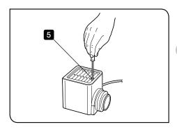
Fit the halogen lamp housing from the above and while pressing down the fixing screw, tighten it with the Allen screwdriver.
