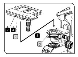
This picture shows the procedure to attach the right hand control 150 mm x 100 mm stage (U-SIC64). The same procedure also applies when attaching other stages.
