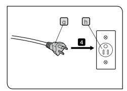
4 Connect the power cord plug g to the power outlet h (Perform this operation for both power cords of the AC adapter connected to the control box and the AC adapter connected to the microscope frame.)
