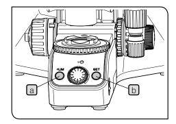
Restoring the stored brightness (LIM function) to the factory default setting
