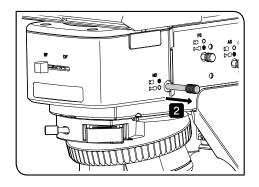
2 Pull out the ND filter lever and remove the ND filter from the light path.
