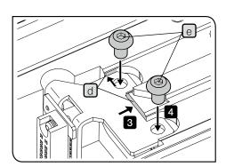
This picture shows the procedure to attach the cable for motorized nosepiece to the microscope frame. The same procedure applies when attaching it to the height adapter.
