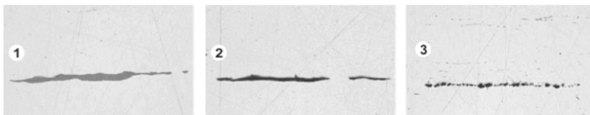
Microscope image of different inclusions in a polished steel sample. The inclusions differ in their color and form. The images show a sulfide inclusion (1), a silicate inclusion (2), and an aluminum inclusion (3).
