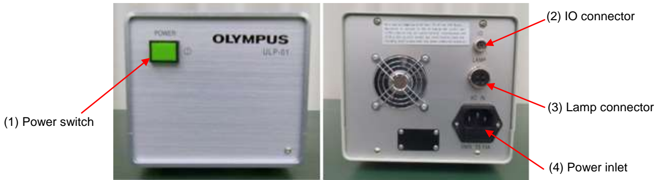
Figure 3. Light source power supply
