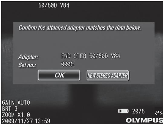
This screen shows the set numbers and adapter names of the stereo optical adapters registered that are the same type as the stereo optical adapter that is connected.
