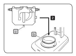
2 Place the stage clamping knob c of BH2-SH (horizontal knob stage) on the front of the base, rotate the clamping knob c in clockwise direction to secure it, and attach BH2-SH.
