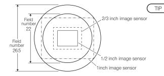
For your reference, the following diagram shows the areas of imaging field determined by the field of view when eyepieces with a field number of 22 or 26.5 are used and the size of the image sensor through the C-mount camera adapter.
