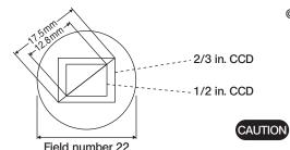
The following diagram shows the areas of the imaging field when eyepieces with a field number of 22 are used for reference. The image field area is determined by the field of view of the eyepieces and the size of the CCD seen through the camera adapter.
