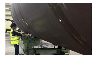
Used in lieu of radiography (RT), our advanced phased array (PA) testing solution using WeldSight software improves the efficiency of piping and vessel weld testing in compliance with ASME, ISO, and similar fabrication codes. Inspect austenitic materials including cladded piping and dissimilar metal welds using our 1D phased array probes, TOFD, and DLA\DMA phased array probes.
