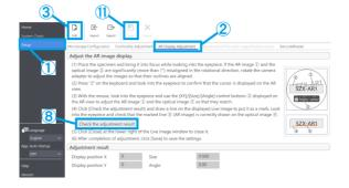
on the AR display to make adjustments so that the AR image (a) matches the optical image (b).
