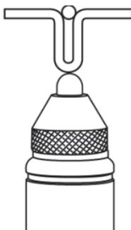
**Figure 4-16 Inaccurate measurement due to surface curvature**
