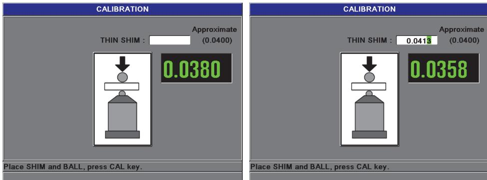
Figure 4-8 THIN SHIM calibration point
