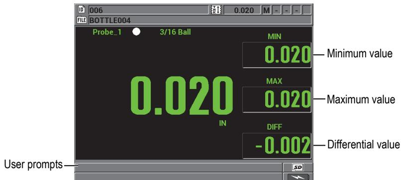
Figure 2-2 Example of other elements appearing on the measurement screen
