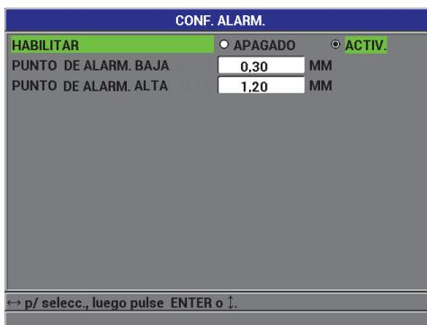
The screenshot shows a screen titled "CONF. ALARM." with a blue header. Below the header, there are two radio buttons: "HABILITAR" (selected) and "APAGADO". To the right of "APAGADO" is another radio button labeled "ACTIV.". Below these are two input fields: "PUNTO DE ALARM. BAJA" with the value "0,30" and unit "MM", and "PUNTO DE ALARM. ALTA" with the value "1,20" and unit "MM". At the bottom of the screen, there is a prompt: "↔ p/ selecc., luego pulse ENTER o ↓".
