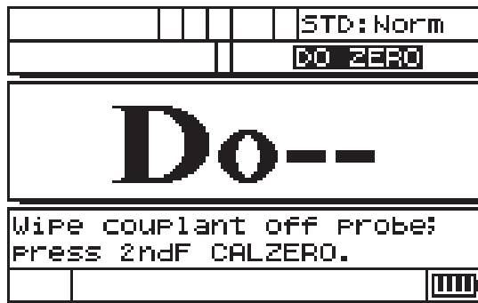
Figure 4-1 Transducer zero compensation
