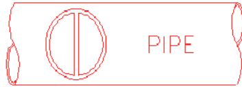
Figure 10-1 Perpendicular to center axis alignment on pipe
