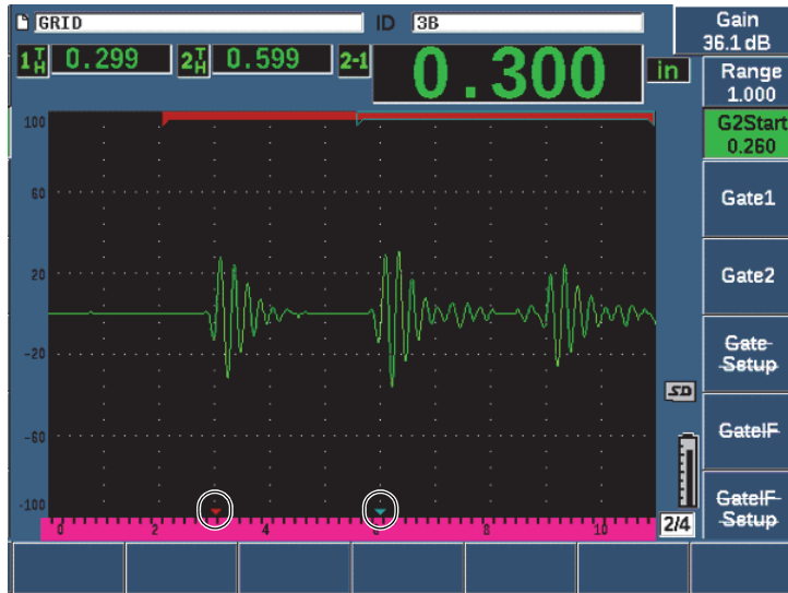
Figure 11-43 Echo measurement error
