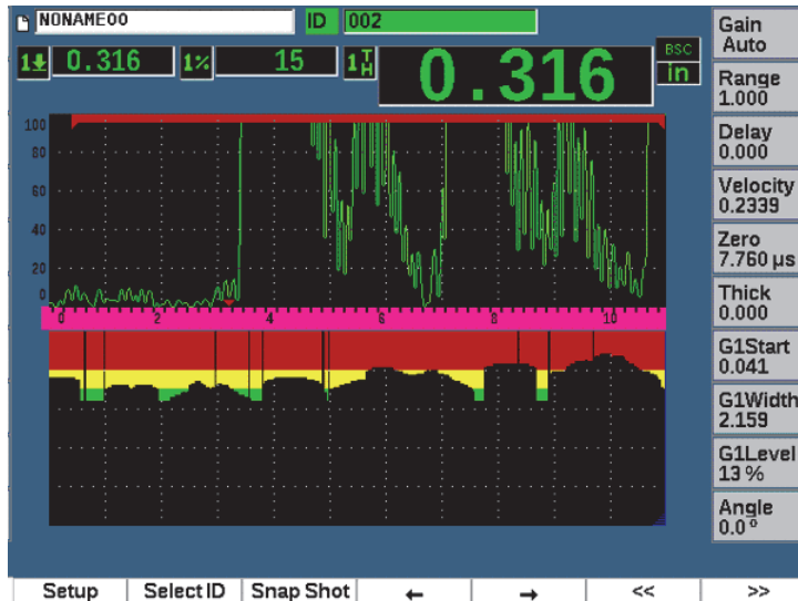
Figure 11-47 B-scan display in the Data Logger
