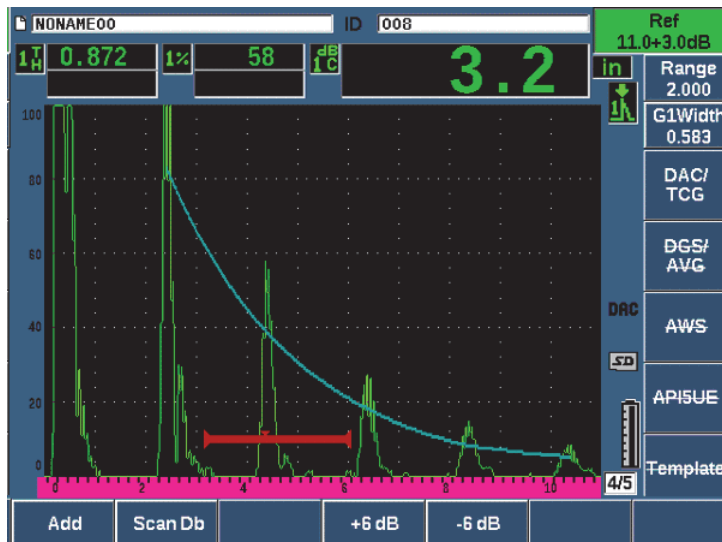
Figure 11-9 Standard DAC with 3 dB scanning gain
