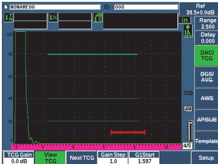
Figure 11-7 Completed DAC curves in TCG view mode
