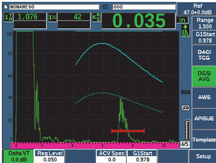
Figure 11-16 DGS/AVG curves on screen
