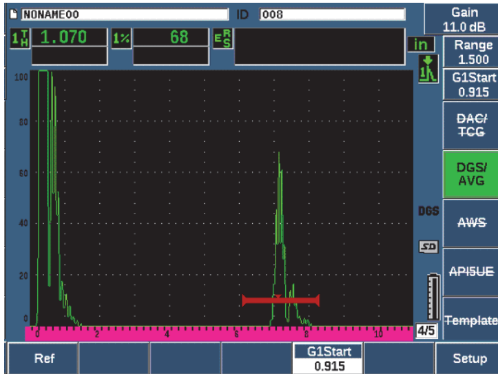
Figure 11-15 Reference-reflector before capture
