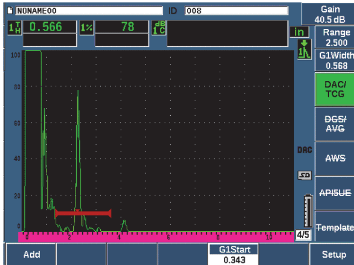
Figure 11-3 First DAC setup step
