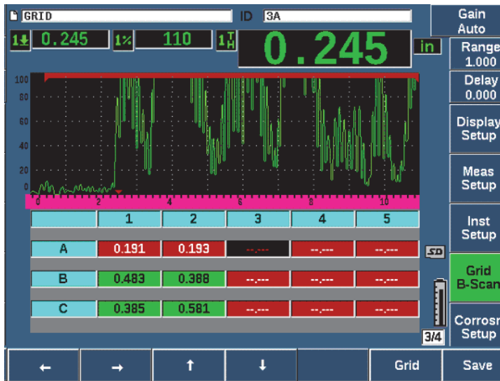
Figure 11-37 Corrosion Module grid view
