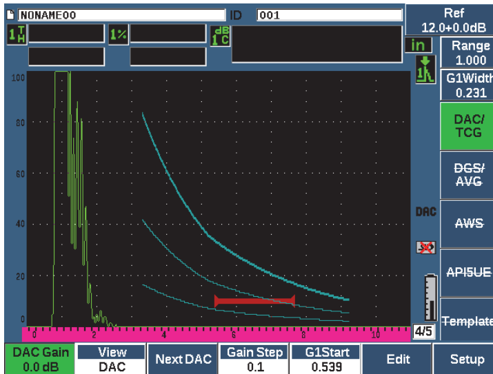
Figure 11-6 The completed DAC curve
