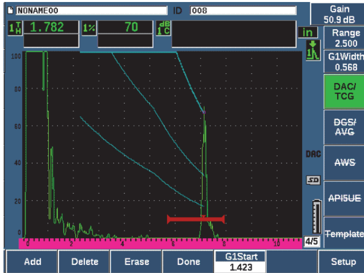
Figure 11-5 Partial DAC curve with each echo set to 80 % FSH
