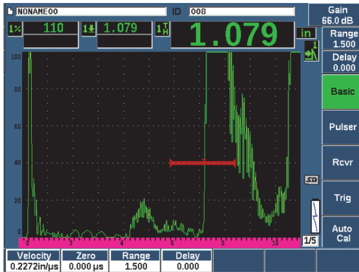
Figure 9-12 Example of a gated signal for velocity calibration
