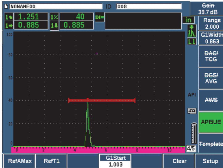
Figure 11-26 Storing the T_1 point
