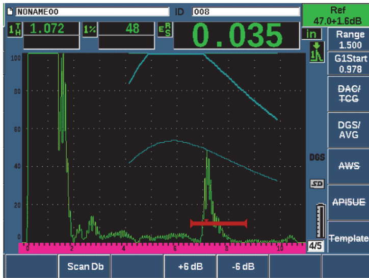
Figure 11-17 Gain curve adjusted DGS
