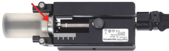
Figure 2-1 Filling the tire chamber with liquid
