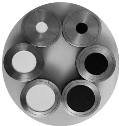
To open the filter holder, rotate the clamp, remove any filter from the desk, place a new filter centrally on the desk.
