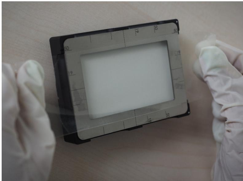
2. Glue the tape to the frame such that the 50 mm wide tape is inside the respective markings. Make sure that the sample is as flat as possible and be careful not to stretch the tape while mounting.
