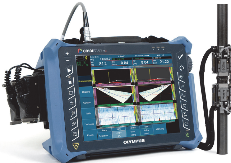
Figure i-1 The OmniScan MX2 and the COBRA scanner
