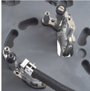
Figure 2-13 Installing the probe holder into the setup template
