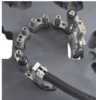
Figure 2-14 Installing male links
