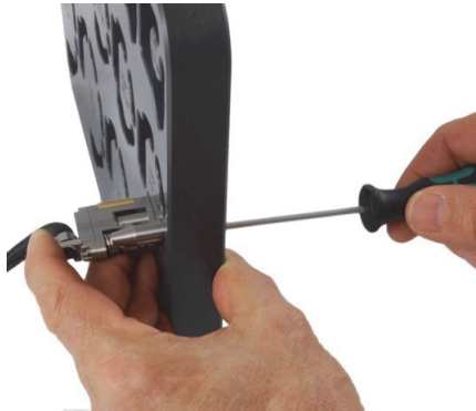
Figure 2-9 Tightening the tail-adjustment screw
