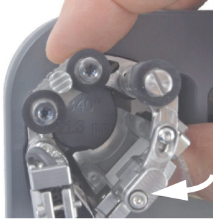
Figure 2-17 Rotating the probe holder to set position for OD smaller than 33.4 mm (1.315 in.)
