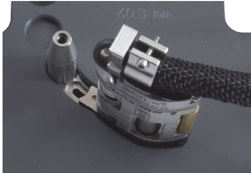
Figure 2-8 Insert the tail in its setup template pocket
