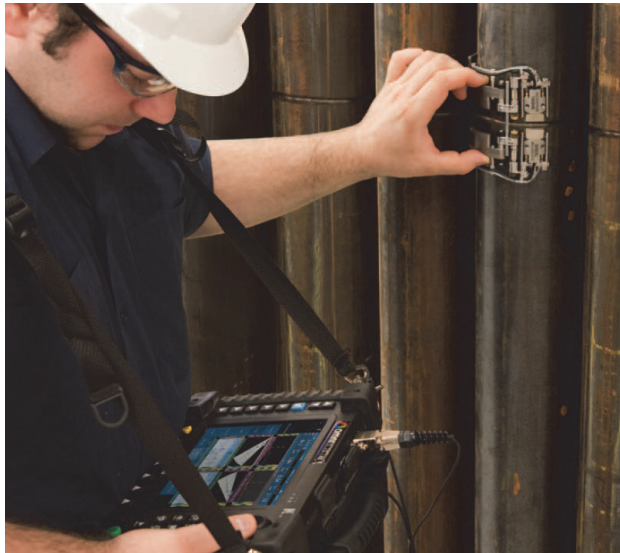
Figure i-2 Operating the COBRA scanner in a limited access area
