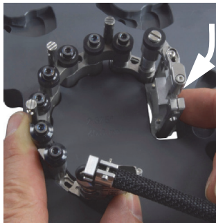
Figure 2-16 Rotating the probe holder to set the position for OD larger than 33.4 mm (1.315 in.)
