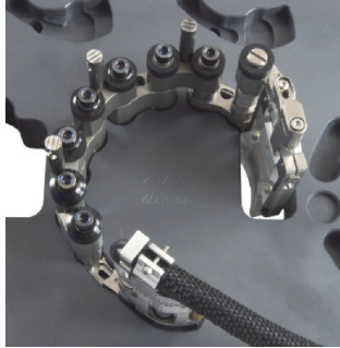
Figure 2-15 Installing female and/or medium links
