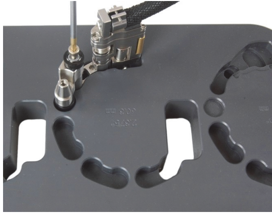
Figure 2-11 Installation du demi-maillon
