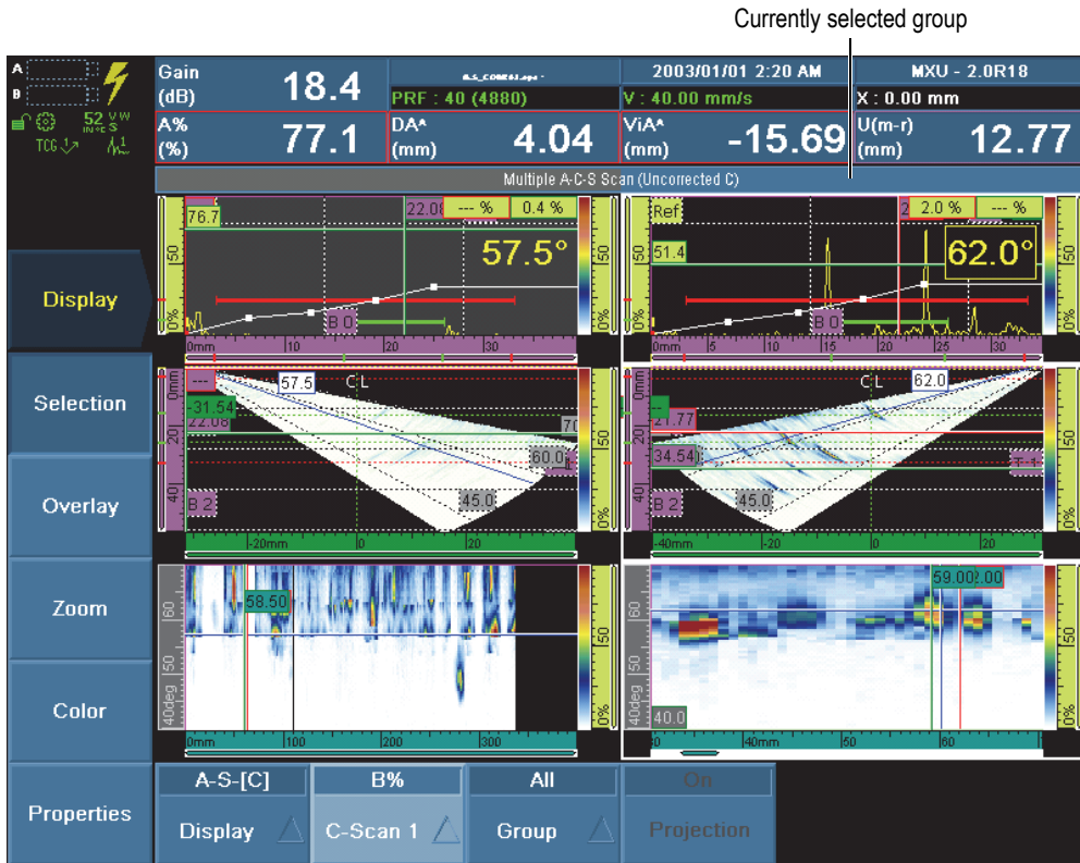
Figure 7 View of A-Scan, S-Scan, and C-Scan for both groups in Analysis mode
