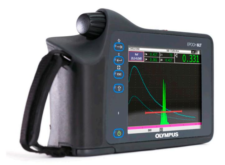
The EPOCH<sup>®</sup> 6LT flaw detector combines ruggedness and ease of use in an instrument designed to be operated using only one hand, enabling fast, efficient rope access inspections and maximum uptime.
