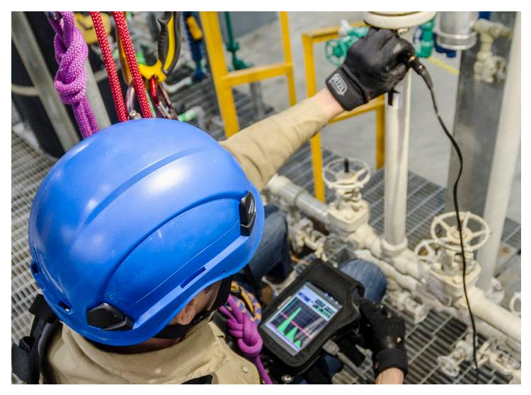
The workflow of the EPOCH<sup>®</sup> 6LT flaw detector is simple and straightforward. The primary screen is a large, optimized A-scan display that contains links to commonly used features and functions. Combined with an improved scanning workflow, users can complete their inspections with minimal button presses and adjustments. When you do need to navigate the menu, prominent icons make it easy to find the feature you're looking for.
