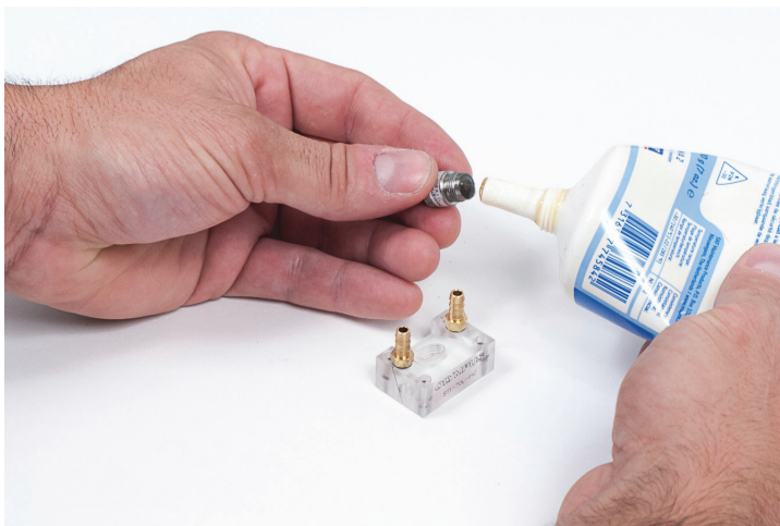
Figure 1-4 Applying couplant on probe face
