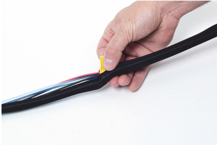
Figure 1-17 Fingers placed under the draw-in tool
