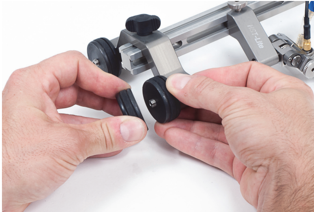
Figure 1-25 Installing an additional wheel
