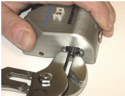
Figure 3-3 Pulling the shaft out of the VersaMOUSE
