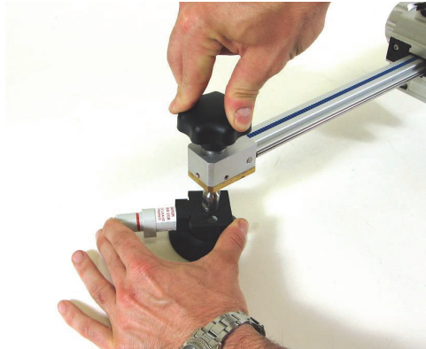
Figure 2-38 Attaching manual suction cups to the inspection surface
