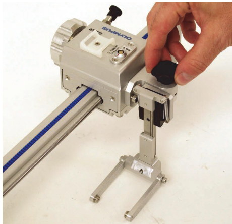
Figure 2-18 Loosening the knob
