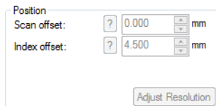
Figure C-6 The Scan axis offset on the Probe tab of the UT Settings dialog box
