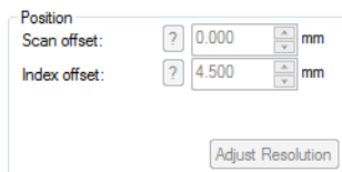
Figure D-4 The Scan axis offset on the Probe tab of the UT Settings dialog box
