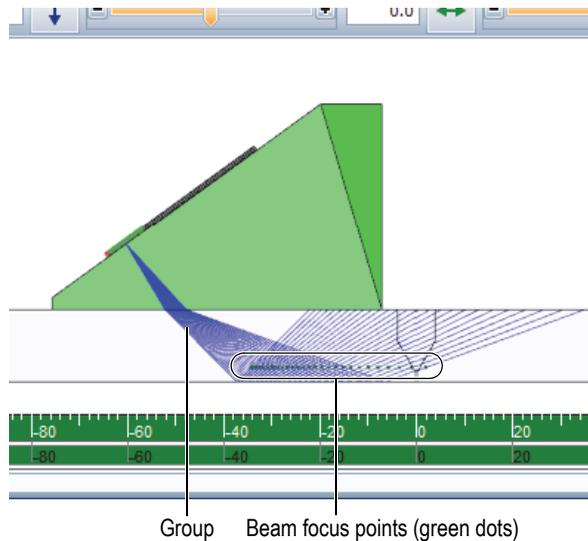
**Figure 10-26 Example of beam focus points represented in RayTracing view**
