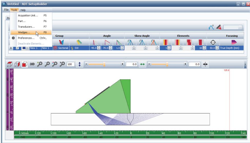
**Figure 9-18** Selecting the Wedges command from the Tools menu
