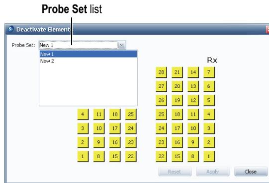
Figure 9-15 The Deactivate Elements dialog box for a dual matrix probe
