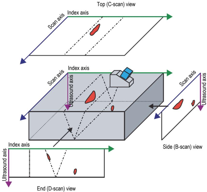
**Figure 4-11 Top, Side, and End ultrasonic views with 90° probe skew angle**
