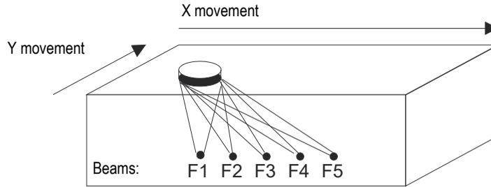
**Figure A-6 Sectorial scanning of X-axis using phased array deflection**
