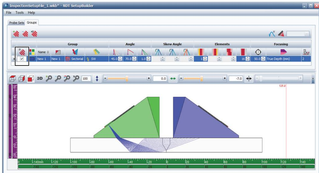
Figure 10-9 The Groups tab with a group's visibility check box selected (in the far-left column)
