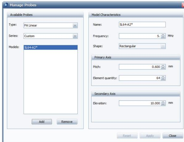
**Figure 9-12** The Manage Probes dialog box and a new probe
