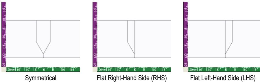
**Figure 8-8 Available weld symmetry options**
