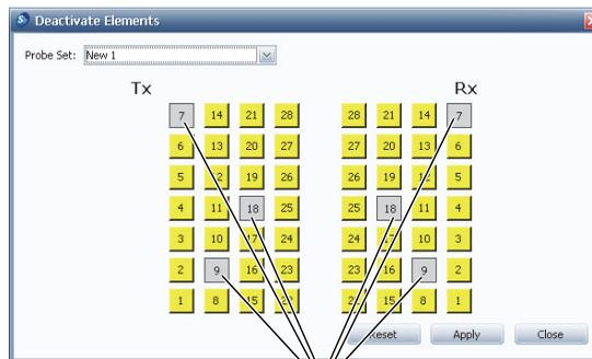
Deactivated elements on the **Tx** and **Rx** matrices**Figure 9-17** The Deactivate Elements dialog box for a dual matrix probe
