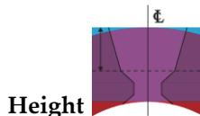
To configure the fill region’s height, enter a value in the **Height** box. This measurement is always taken parallel to the weld center line.
