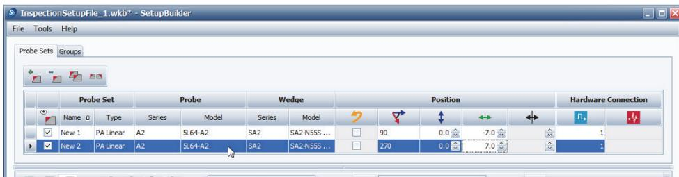
Figure 9-6 Selecting a probe set on the Probe Sets tab to configure parameters
