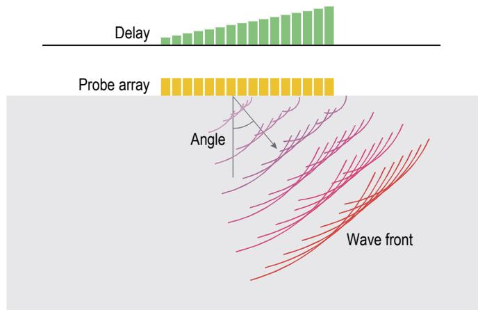
**Figure A-3 Ultrasonic beam angle control of a linear array**
