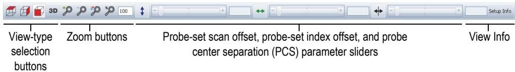
**Figure 4-13 The toolbar for the RayTracing view**
