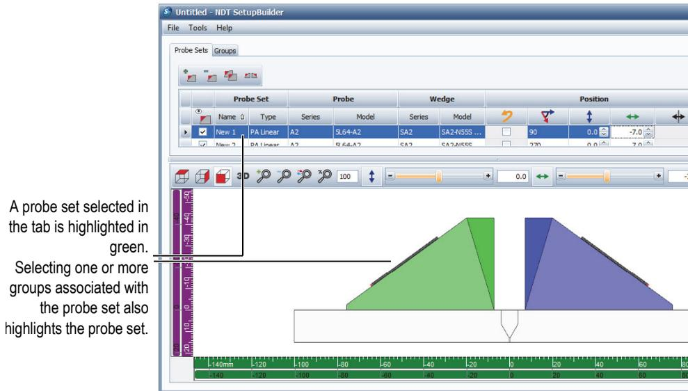
Figure 4-3 The selected probe set highlighted in green in RayTracing view
