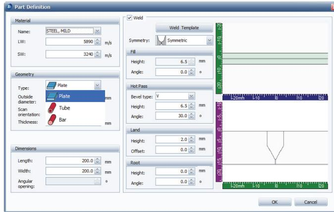
Figure 8-3 The Type list in the Part Definition dialog box
