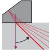
**Figure 10-15 Refracted angle start measurement**
