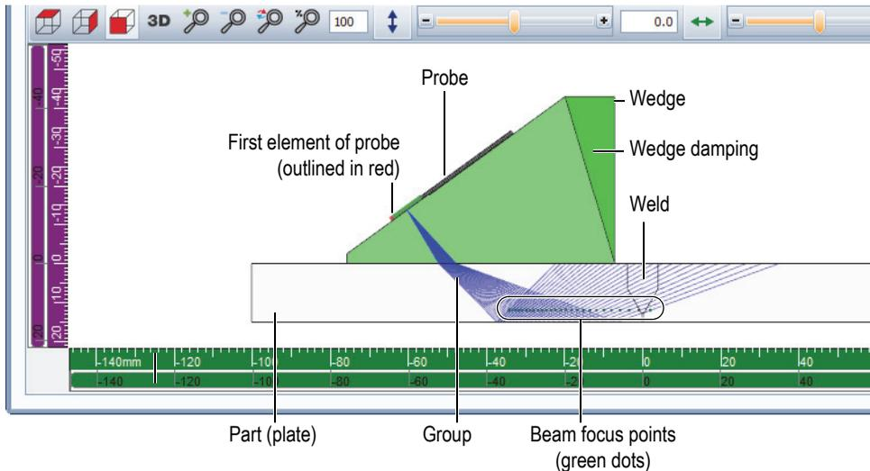
Figure 4-15 Part, weld, probe set, and group representation in RayTracing view
