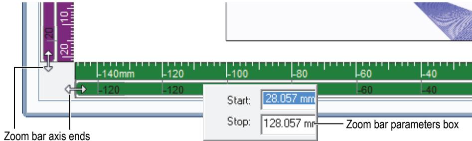
Figure 4-21 Zoom bar controls in RayTracing view
