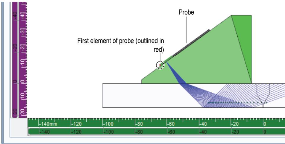
Figure 9-9 The first element of a probe is identified in RayTracing view
