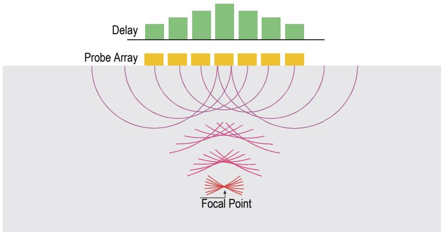
**Figure A-4 Ultrasonic beam focusing of a linear array**
