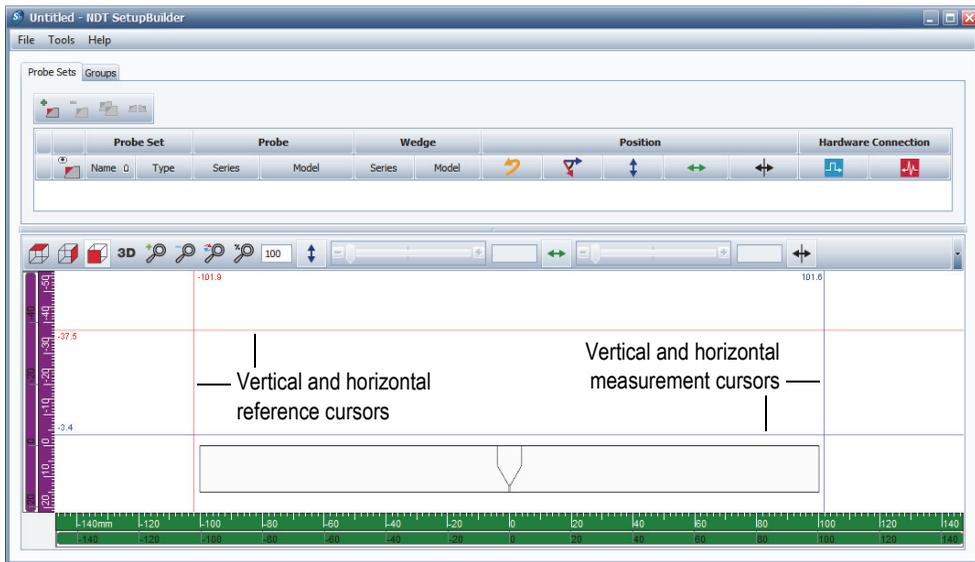
Figure 4-22 Reference and measurement cursors in RayTracing view
