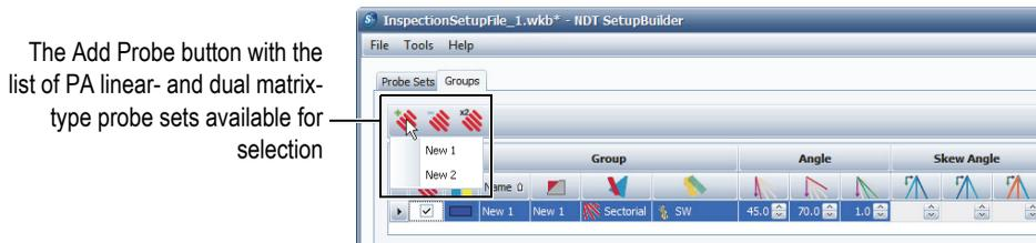
**Figure 10-2** The Add Probe button with the Probe Sets list displayed
