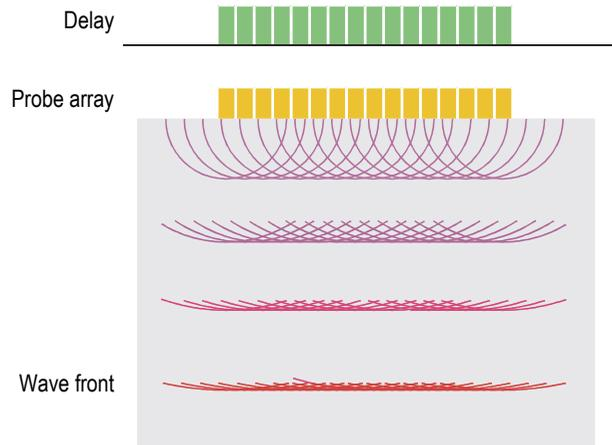
**Figure A-2 Ultrasonic wave front of a linear array**
