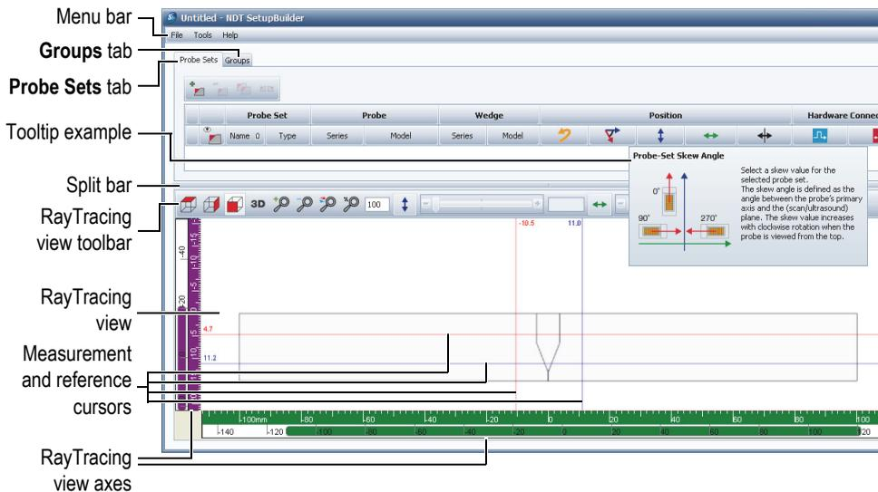
**Figure 4-1** The NDT SetupBuilder user interface
