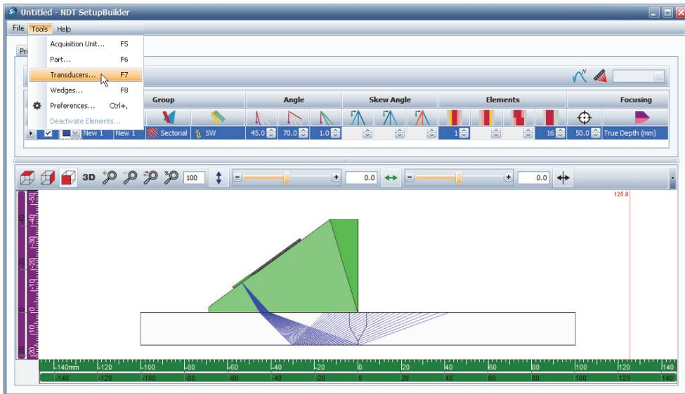
**Figure 9-10** Accessing the probe settings on the Tools menu
