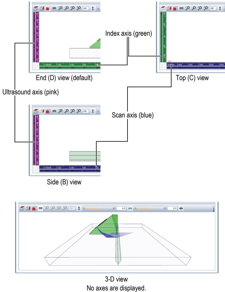
**Figure 4-12 Axis content for the RayTracing view options**
