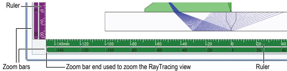
**Figure 4-14 RayTracing view axis components**
