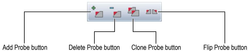
**Figure 9-1 The Probe Sets tab toolbar**
