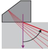
**Figure 10-16 Refracted angle stop measurement**
