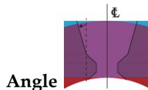
To configure the wall angles of the fill region, enter a value in the **Angle** box. The fill angle is defined as the angle between the fill bevel and a line parallel to the center line.
