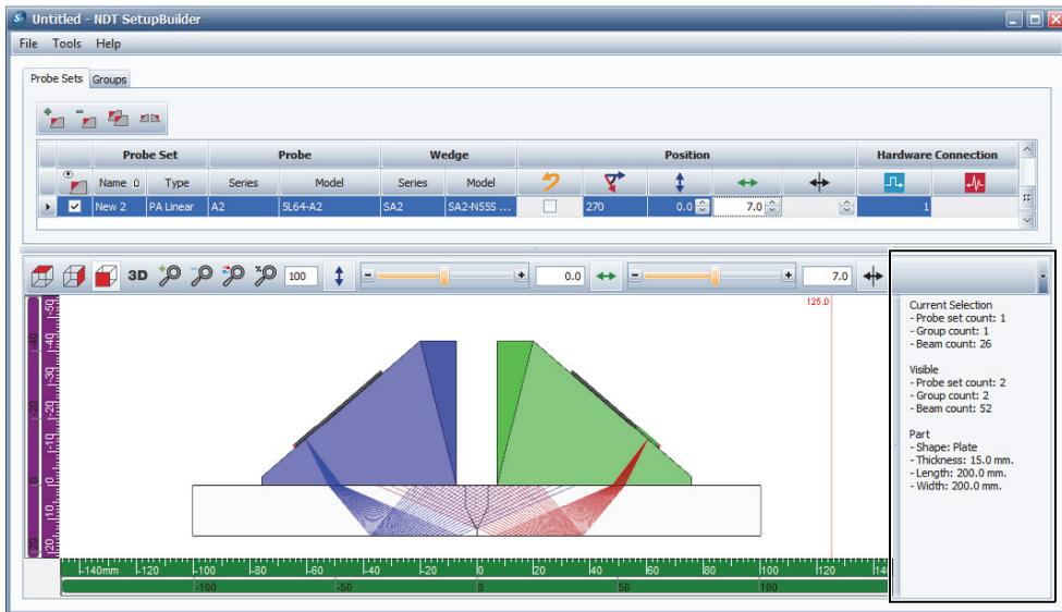
Figure 4-20 The RayTracing view with the Setup Info pane displayed
