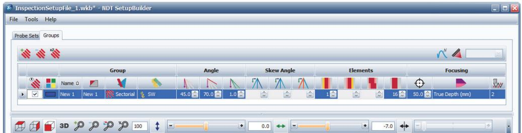
Figure 10-7 Setting the beam-formation visibility on the Groups tab
