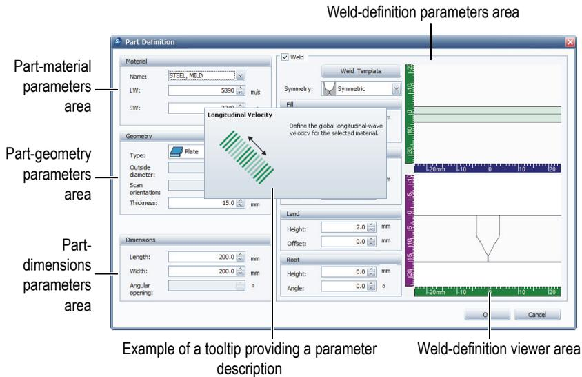
**Figure 8-2 The Part Definition dialog box with default parameters**
