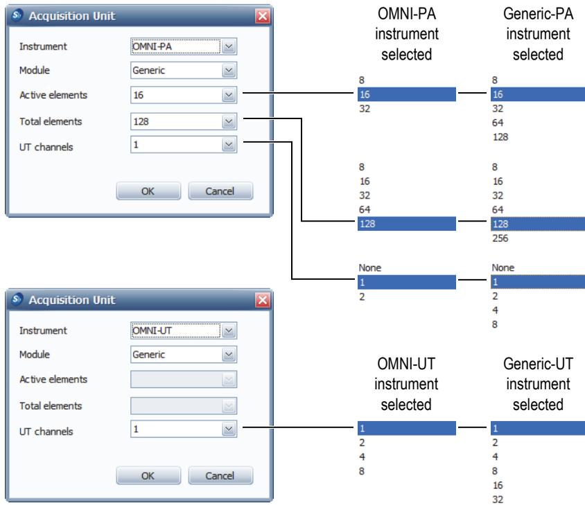
**Figure 7-3** The Acquisition Unit dialog box with the various list options
