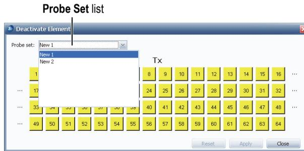
Figure 9-14 The Deactivate Elements dialog box for a PA linear probe
