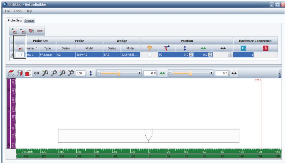
Figure 9-8 A probe set with the Visibility check box cleared on the Probe Sets tab
