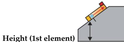
Enter a value indicating the height (tertiary offset) of the middle of the first reverse element of the probe-set probe relative to the material surface, with a 180° orientation on the wedge (see Figure 9-22 on page 128).
