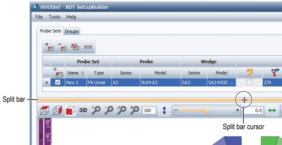
Figure 4-23 Using the split bar to modify the size of the main window's panes
