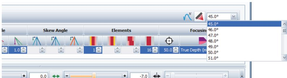
Figure 10-8 Selecting the displayed beam in the Active Beam list
