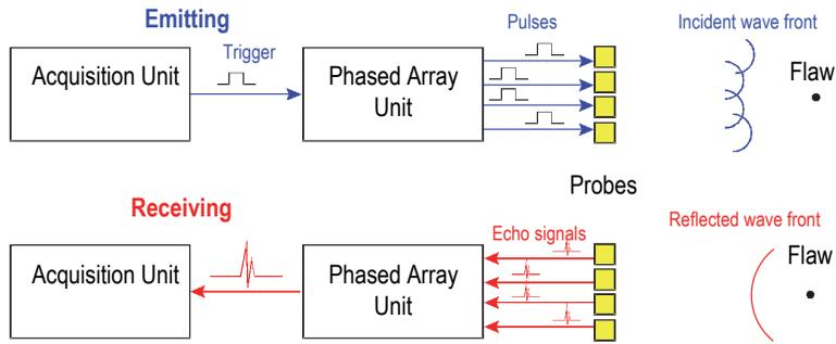
**Figure A-1 Emitting and receiving in a phased array system**
