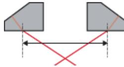
Figure 9-27 Probe center separation measurement
