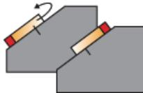
**Figure 9-23** Example of a probe mounted backwards on a wedge
