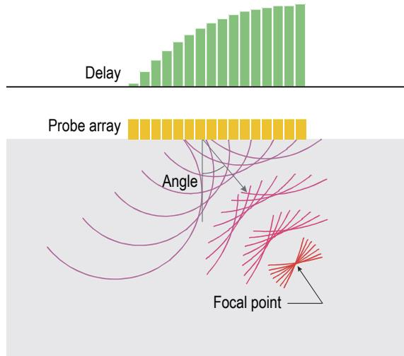
**Figure A-5 Ultrasonic beam angle control and focusing of a linear array**
