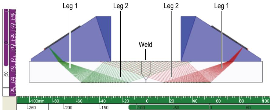
**Figure 10-29 The legs for groups of two probe sets with 90° and 270° skew angles**
