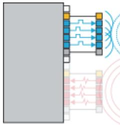
**Figure 9-28 Pulsing probe with first element marked in yellow**
