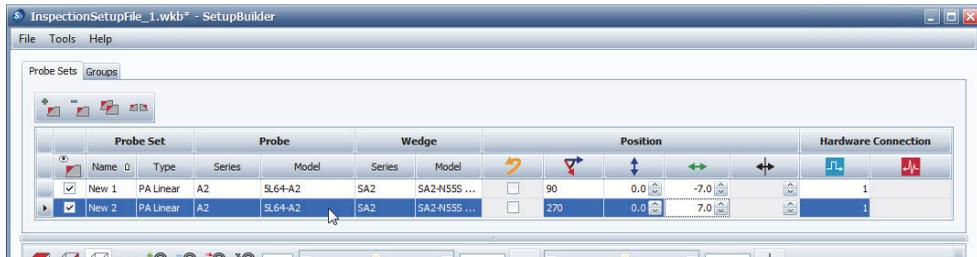
Figure 9-4 Selecting a probe set on the Probe Sets tab for flipping
