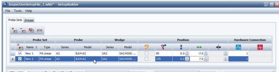
**Figure 9-2** Selecting a probe set on the **Probe Sets** tab for deletion
