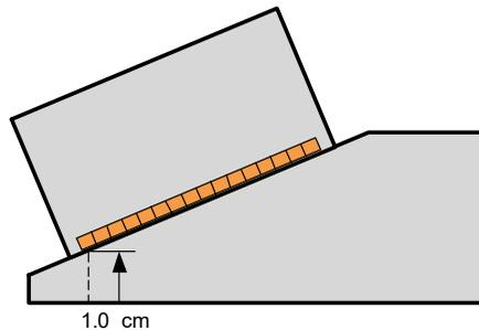
Figure 9-22 The height of the first element
