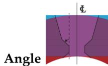
To configure the wall angles of the hot-pass region, enter a value in the **Angle** box. The hot-pass angle is defined as the angle between the hot-pass bevel and a line parallel to the weld center line. The maximum usable value for the hot-pass region wall angle is  $89.9^\circ$ , and the minimum height value is 0.0 mm. A hot-pass height value of 0.0 mm means that no hot pass is defined. A minimal value greater than  $0.0^\circ$  is needed to define the hot pass angle.
