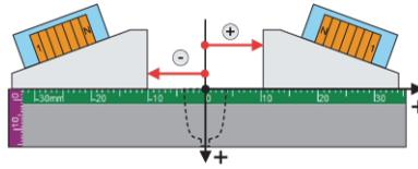
Figure 9-26 Probe-set index offset
