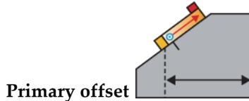
Enter a value indicating the primary axis offset of the middle of the first reverse element of the probe-set probe relative to the back of the wedge, with a 180° orientation on the wedge. The offset is always measured along a straight line, and normally has positive values.
