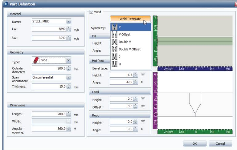
**Figure 8-10 The Weld Template list**
