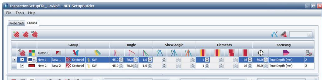
Figure 10-12 Selecting a group on the Groups tab for configuring parameters
