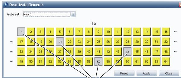
Deactivated elements on the **PA** linear matrix**Figure 9-16** The Deactivate Elements dialog box for a PA linear probe
