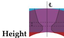
To configure the hot-pass region’s height, enter a value in the **Height** box. This measurement is always taken parallel to the weld center line.
