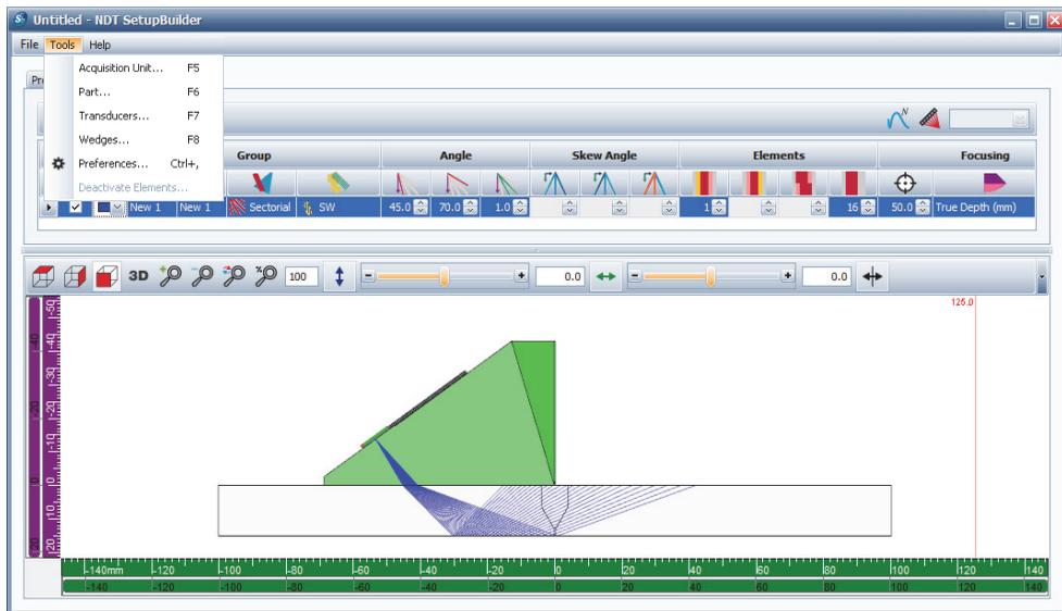
Figure 8-1 Default plate part with simple symmetrical V weld in RayTracing view
