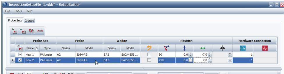
Figure 9-3 Selecting a probe set on the Probe Sets tab for cloning
