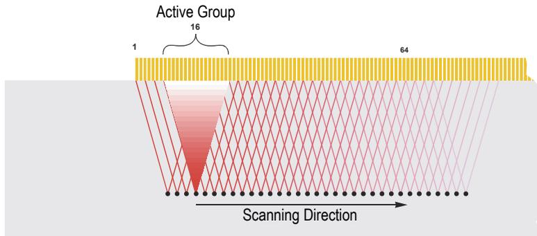
**Figure A-7 Electronic scanning along an axis**
