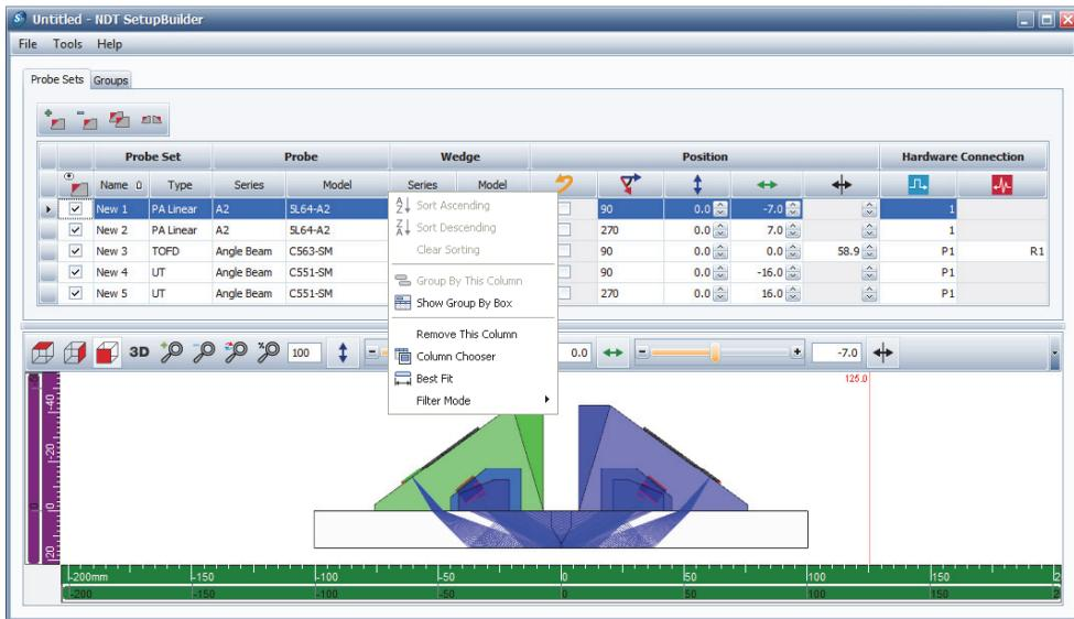
Figure 4-7 Removing a column from a tab
