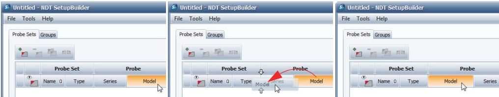
Figure 4-4 Dragging a column header on a tab
