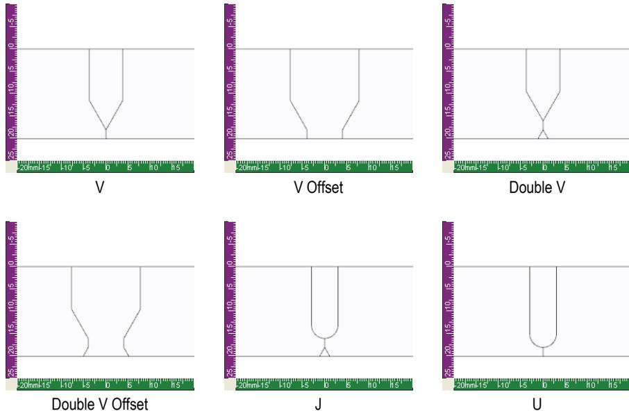
**Figure 8-7 Available weld shape templates**
