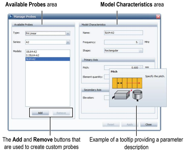
**Figure 9-11 The Manage Probes dialog box**
