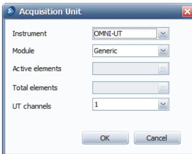
Figure 7-2 The Acquisition Unit dialog box with UT target technology
