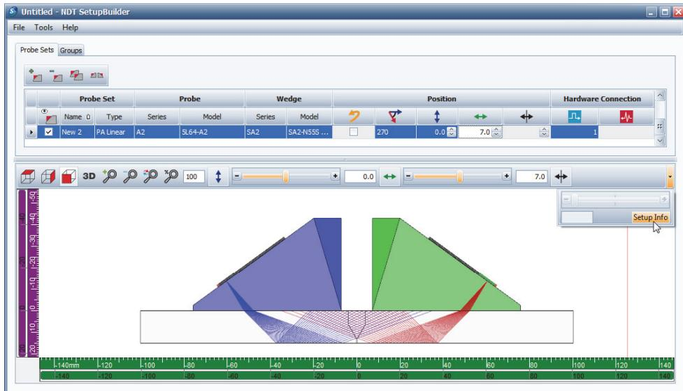
**Figure 4-19** Clicking the Setup Info button on the RayTracing view toolbar
