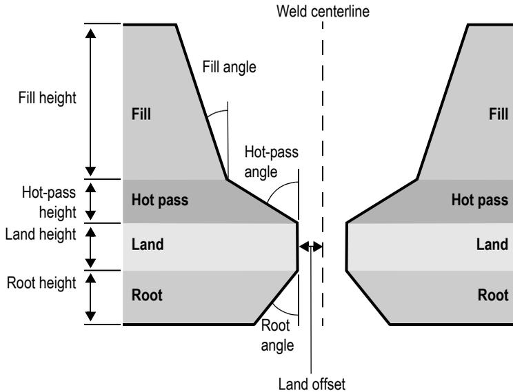
**Figure 8-5 The parts and parameters of a weld definition**
