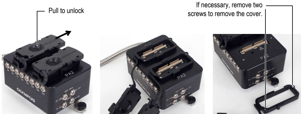
Figure 2-8 Removing the PA protective covers
