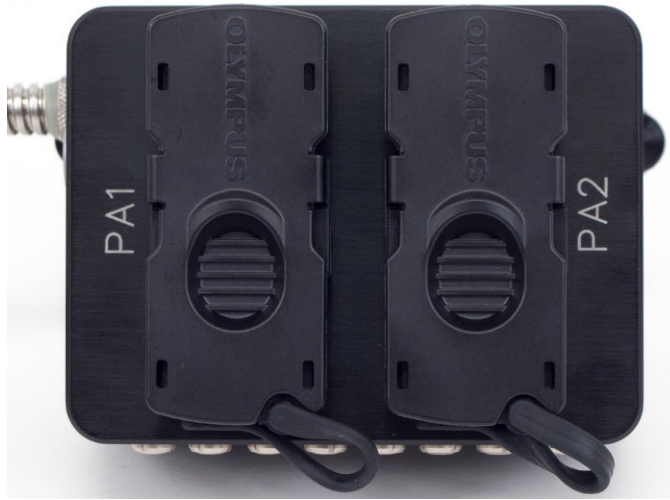
Figure 2-7 The protective covers for phased array connectors (PA1 and PA2)
