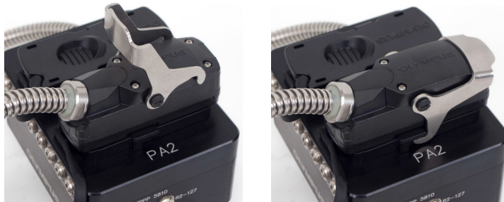
Figure 2-10 The OmniScan connector pushed in ( left ) and locked ( right )
