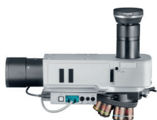
2. BX3M-RLA-S Reflected light illuminator for BF/DF
